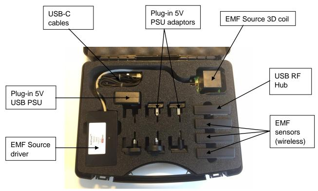
EMF Source driver: The EMF Source driver is hardware to the EMF Source coil, and powered from 5V through USB port or by using the 5V USB wall plug-in adaptor supplied with the system. Communicating with EMF sensors and USB RF hub is done using 2.4GHz proprietary RF link.
