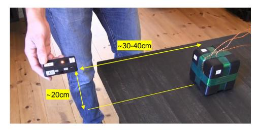
When the correct calibration position is found, the sensor LED will stop flashing yellow and light up constantly yellow. Then push the sensor button, and if start up calibration is successful, the LED turns green, and the sensor should now be visible in the AmfiTrack Viewer software.
